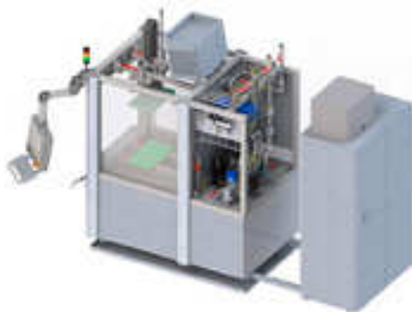
Schaltschrank in Servicestellung Cabinet in service position
