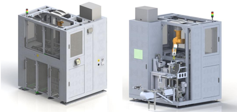
6-axes-robot, 2 trolley boxes and measurement system
